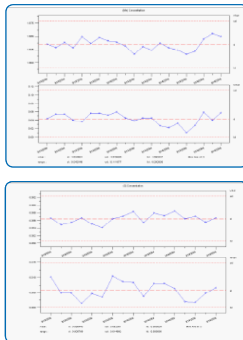
Measurements over a couple of days show significantly low deviations. Charts of Q8 Magellans database software show moving averages and ranges of Manganese and Sulphur.
